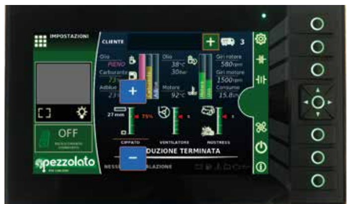
Electronic controller with 7" "touch screen" panel
