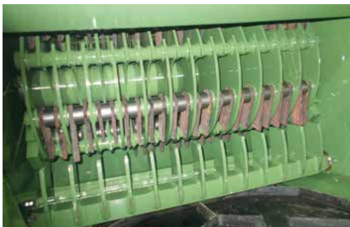
S 9000 rotor with moving hammers and counter-hammer
