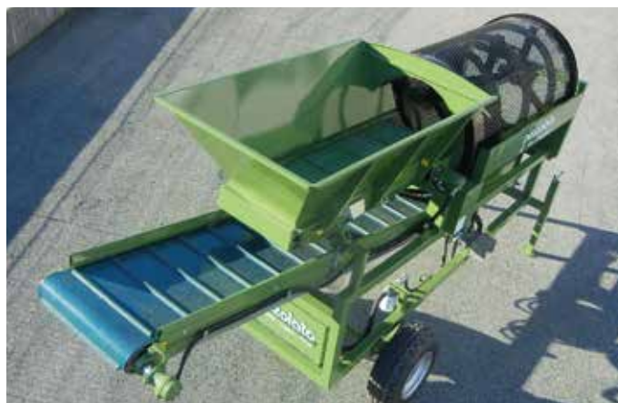
Material discharge belt under screen
