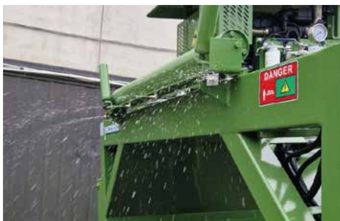
Two-inch ramp for liquids distribution
