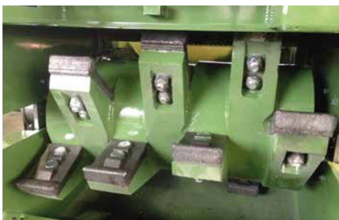
MF 10000 rotor with fixed hammers
