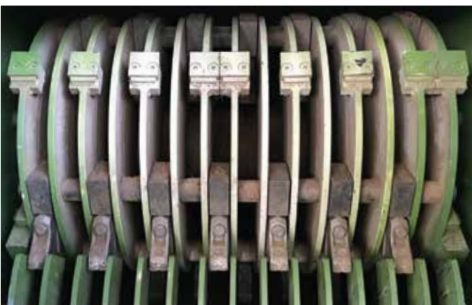
S 10000 rotor with movable hammers and counterblade
