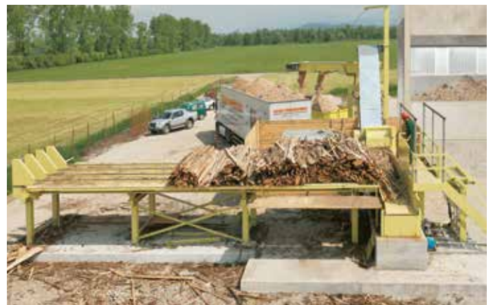
Loading decks with 4 chains for logs and slabs
