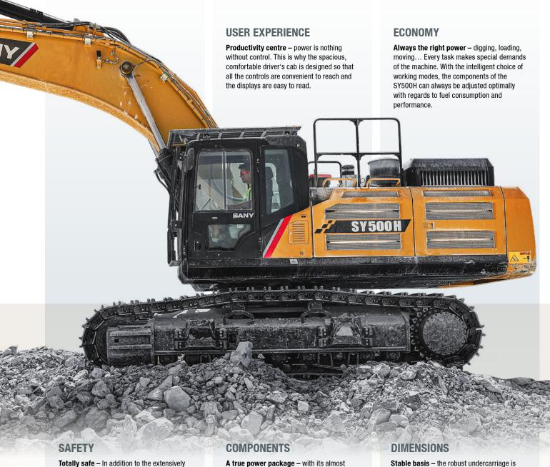
glazed driver's cab, the standard rear camera guarantees excellent visibility on all sides with no blind spots. The reinforced cab structure in accordance with ROPS/FOPS specifications ensures a safe work environment for the machine operator.
