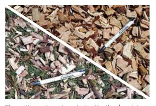
The cutting system characterized by the closed drum and the interchangeable calibration grid according to the needs, allow to obtain a uniform and homogeneous wood chips even from material of little value.
